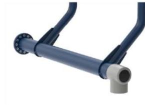
The input shaft is Ø101,3 x 2,9mm S355 Hot Dip Galvanized and Powder-coated steel. The bearing house is Cast Aluminum (EN AB-44100 / EN AB-AISI12(a)) with self-aligning sealed ball bearings. An extremely strong and durable construction.
