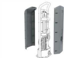
The cover protects all the moving parts from vandalism and entrapments. The cover is made of 5mm rotomolded LLDPE, Linear low-density polyethylene, with excellent impact strength and usable within a large temperature span.
