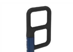
The ergonomically shaped handles have different grip areas for adaptable training, allowing people from 140 – 205 cm tall, to perform the exercise ergonomically correctly and at the same time allowing multiple different exercises. The handles are Aluminum cast and have a diameter of  $\varnothing$  33mm. The Grip Powdercoating, used on the support handle, is highly durable against wear and tear, offers isolation, and simultaneously gives users an outstanding grip
