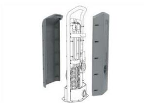
The cover protects all the moving parts from vandalism and entrapments. The cover is made of 5mm rotomolded LLDPE, Linear low-density polyethylene, with excellent impact strength and usable within a large temperature span.
