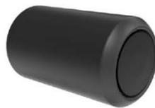
The rotating rollers are  $\varnothing 110$ mm and made from PUR (Polyurethane Rubber, compact foam). The rollers have a steel insert that is electro galvanized. They provide support and ensure a comfortable position.
