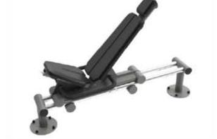
The seat and head support are made of Polyurethane Rubber and have a steel insert plate that connects it to the steel frame. The seat is adjustable in 14 different settings to fit users from 140/205 cm tall and to vary the type of exercises. The seat is positioned under a 12-degree angle and the back supports a 48-degree angle. The back support has a groove, accommodating a comfortable position.
