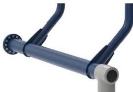
The input shaft is  $\varnothing$ 101,3 x 2,9mm S355 Hot Dip Galvanized and Powder-coated steel. The bearing house is Cast Aluminum (EN AB-44100 / EN AB-ALS12(a)) with self-aligning sealed ball bearings. An extremely strong and durable construction
