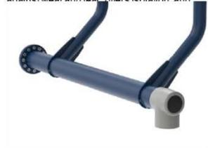
The input shaft is  $\varnothing$ 101,3 x 2,9mm S355 Hot Dip Galvanized and Powder-coated steel. The bearing house is Cast Aluminum (EN AB-44100 / EN AB-AISI12(a)) with self-aligning sealed ball bearings. An extremely strong and durable construction
