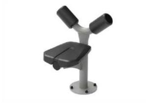
The seat is made of Polyurethane Rubber and has a steel insert plate that is electro-galvanized. The steel plate connects the seat to the frame. This construction makes the seat extremely durable against wear & tear and still very comfortable for a great user experience. The seat is positioned at a height of 46 cm, a comfortable height that makes the transfer from a wheelchair easy.
